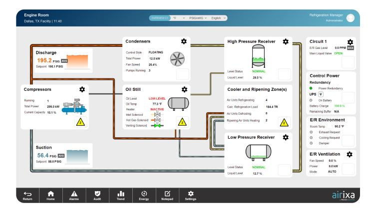
Refrigeration systems need to reliably operate 24/7 to prevent the loss of perishable food products. With Airixa's included supervisory control and data acquisition (SCADA) software, companies can monitor the status, health and performance of their entire refrigeration system from both the plant and enterprise level.
